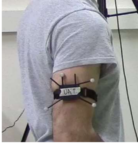
Figure 4.2. IMU and its associated marker cluster attached to the upper arm of a participant
