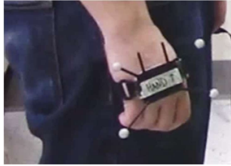
Figure 3.2. IMU and its associated marker cluster attached to the hand of a participant
